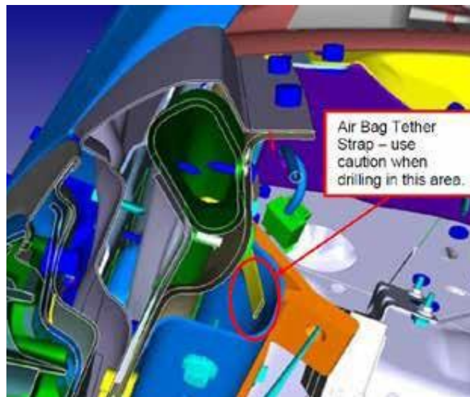
Figure 2: A-Pillar Cross Section
