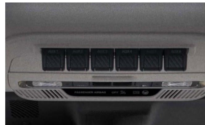
The Ford Upfitter Switches are optional overhead console mount switches (Option Code 66S) that control underhood mounted relay. (Reference the Upfitter Relay Box section of this BBLB). All fuse are in the Upfitter Relay Box.
